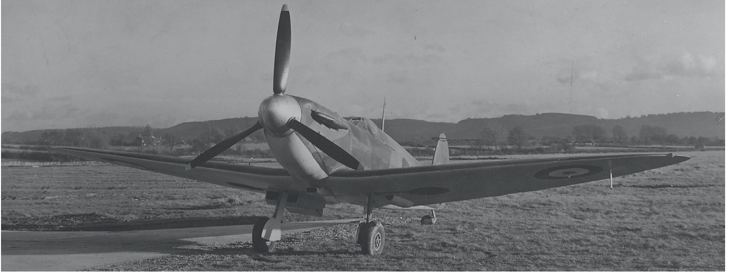
Early built Spitfire Mk.I, already with three-blade De Havilland 5/20 two pitch propeller, late style antenna mast and Pitot tube, but still without armor and gun-heating, still equipped with iron sights. Note the tailplane device, protecting the vertical stabiliser in case of use anti-spin parachute.
